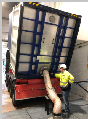
Direct unloading into a bunker
