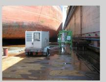
Semi-portable vacuum extraction unit units for water-jetting tools. Separates liquids from solids during operation.
