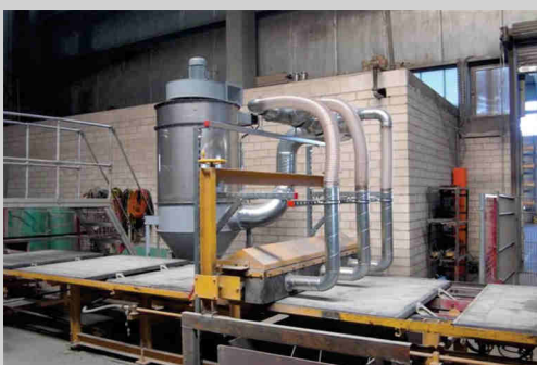
Dust extraction of a brush station for product palettes
